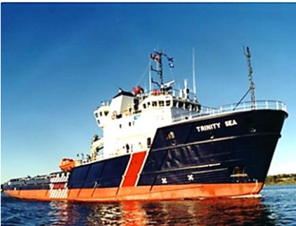
Trinity Sea and Burin Sea built 1983 and rebuilt 1999; the initial trip on the Trinity Sea to the Grand Banks was a frightening experience; heavy bottomed she had a quick five second roll; the crew stood by in the mess waiting for the order to abandon when the roll became extreme (15 degrees each way rail to rail every five seconds) in rough weather; on return to port she was fitted with bilge keels which reduced the extent of
