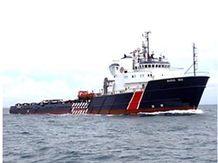
Trinity Sea and Burin Sea built 1983 and rebuilt 1999; the initial trip on the Trinity Sea to the Grand Banks was a frightening experience; heavy bottomed she had a quick five second roll; the crew stood by in the mess waiting for the order to abandon when the roll became extreme (15 degrees each way rail to rail every five seconds) in rough weather; on return to port she was fitted with bilge keels which reduced the extent of
